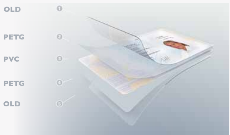
Fig. 4 D2T2 Colour Printable - PETG/PVC Core Card
