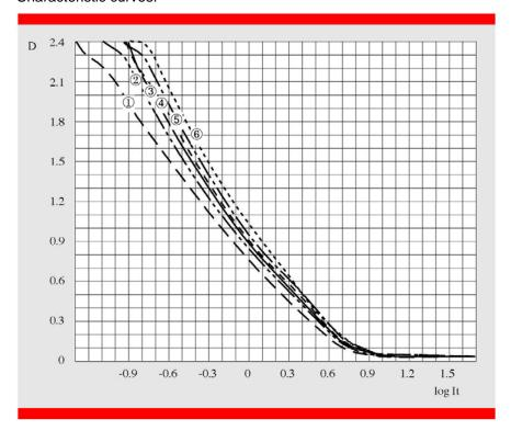
Processed in Gevatone 66, in G 74 c developer at 30  $^{\circ}$ C. Exposure 3500 $^{\circ}$ K, 53 lxs, 21 step wedge.
