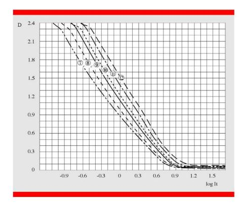
Processed in Gevatone 66, in G 74 c developer + AD 74 at 30  $^{\circ}$ C. Exposure 3500  $^{\circ}$ K, 53 lxs, 21 step wedge.
