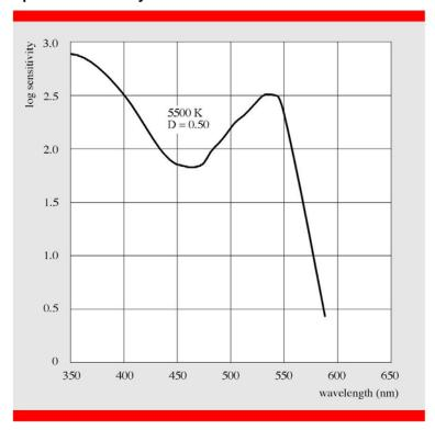
Sensitivity is reciprocal of the exposure  $(mJ/m^2)$  required to produce the indicated density. Developed in Gevatone 66, G 74 c developer, 30 °C for 42 s.
