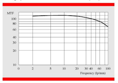
Developed in Gevatone 66, in G 74 c developer at 30 °C, for 20 s (gamma 1.00).
