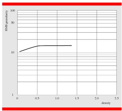
Measured with a spot size of 50  $\mu m$  in diameter. Processing in Gevatone 66, in G 74 c developer, at 30°C and gamma 1.00.
