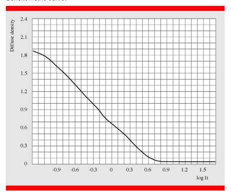
• Processing in Adaptol developer, at 20 °C, for 2 - 4 minutes.
