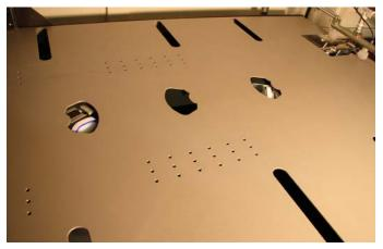
The combination of the patented FlexWheel® and FlexPin® components ensures a perfect, fully automatic and formatindependent 3-point registration of each plate.
