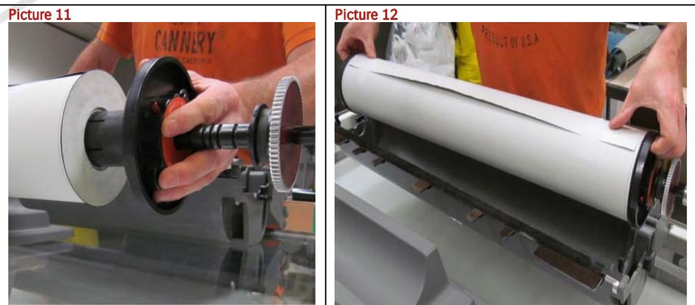
Mount the endcaps of the supply cassette onto the roll core (picture 11).
