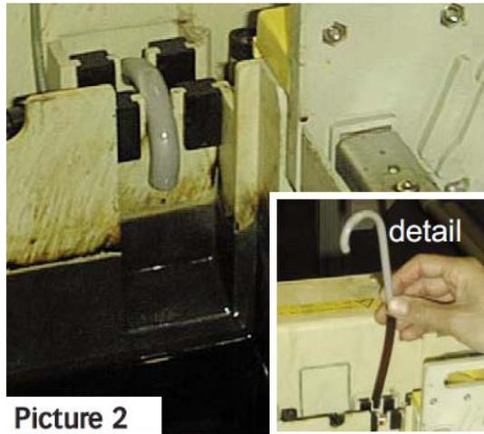
3. Take out the plastic pipe from this fitting and lift it up. (see picture 2)
