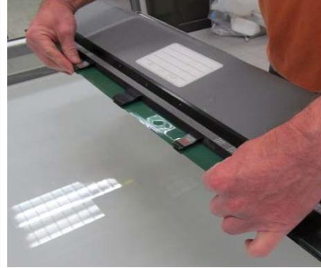
Separate the leader from the film (picture 16 and 17). **Rewind manually** and position the film into the loading position: in line with the front side of the cassette (picture 18).
