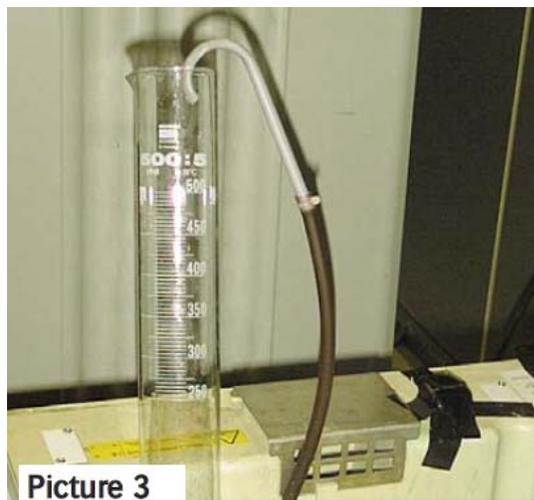
4. Hook the replenishment pipe in a 500 ml measuring glass to enable accurate readings (see picture 3). Make sure the replenishment tank is at least half full. If not it might be impossible to pump up the required quantity.
