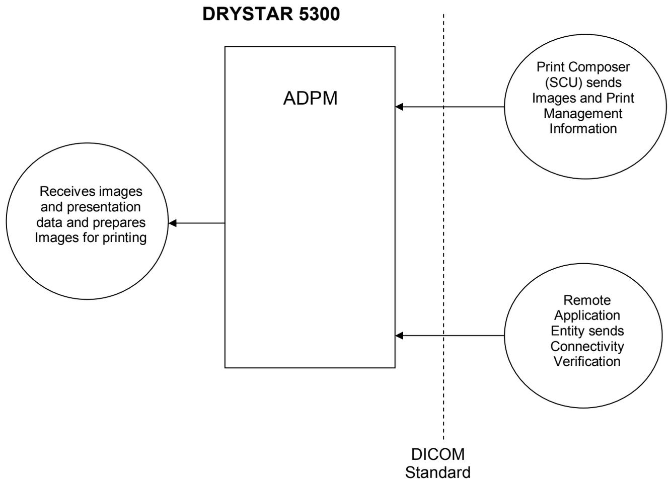
*Figure 2.1-1: Functional Overview – Application Data Flow*
