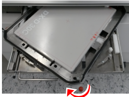
Figure 111: Example: rotate clockwise to change from portrait to landscape position
