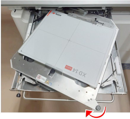
Figure 104: Example: rotate clockwise to change from portrait to landscape position
