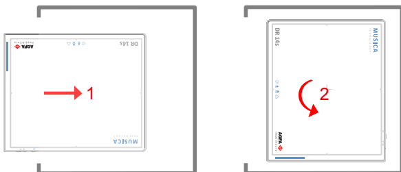
Figure 14: Portrait orientation in the radiographic wall stand left loading
