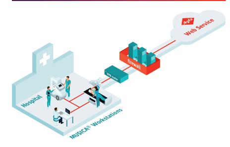
MUSICA® Analytics collects log files from each MUSICA® workstation and transfers them to a secured cloud, where the analytics calculations are performed. Strongly encrypted network communication is used, via a direct connection with the Agfa Web Service (with or without a VPN).
