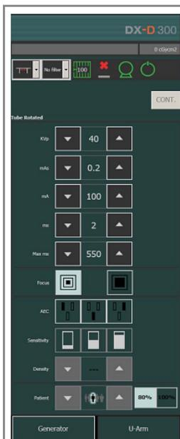
**Figure 4: X-Ray generator controls**
