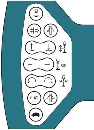
Figure 11: DR Detector handle control buttons
