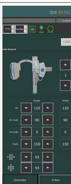
**Figure 5: X-Ray system automatic positioning controls**
