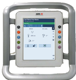
Figure 4: Control Panel of the X-Ray Tube Stand with tube head display (controls for X-ray tube position and for X-ray exposure parameters)
