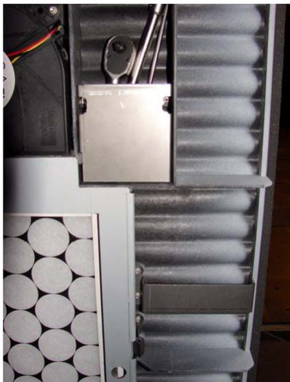
8. Insert the tool in the opening and turn the screw counterclockwise, until the digitizer is lifted up approximately 1,5-2 cm, until you encounter resistance.
