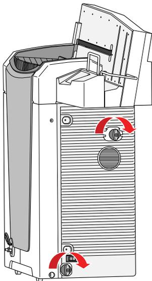
**Table 2: Locked and unlocked position of the handles**
