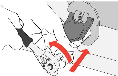
3. On the right side of the digitizer, turn the two handles 180° counterclockwise till they reach the unlocked position:
