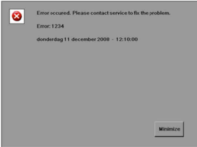
**Figure 7: Example fatal error (status indicator continuously red)**
