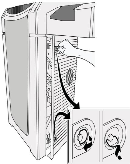
4. Open the right side door and locate the air-filter element inside the door opening.
