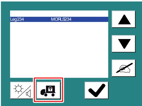
3. Wait for the following message to be displayed: "Ready to fix transport locks. Switch off the digitizer and fix transport locks."
