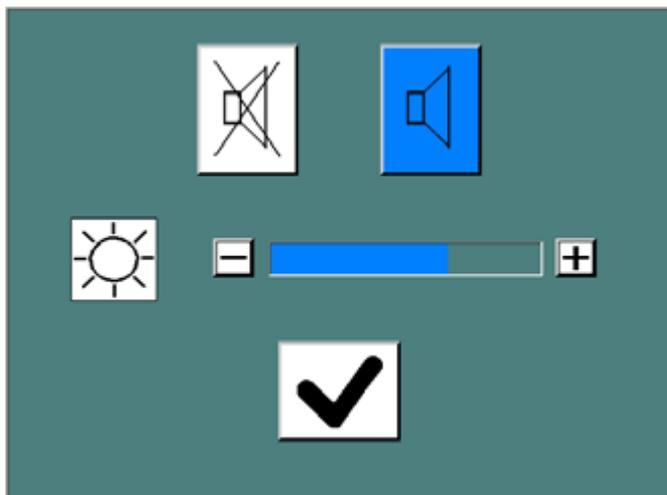
3. In the Brightness section on the lower part of the Configuration window, use the + or - buttons to adjust the brightness.
