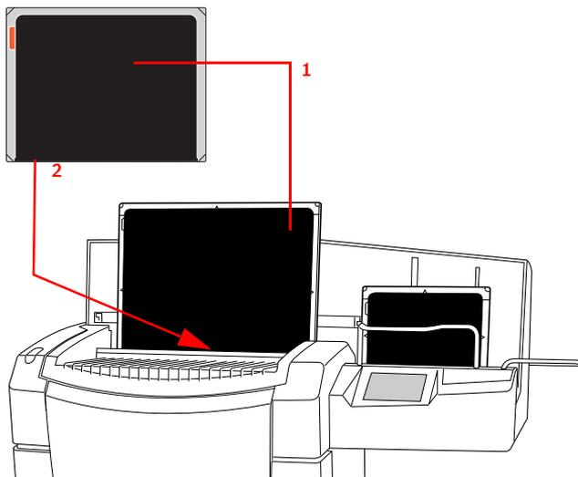
1. Tube side must be faced to the operator.
