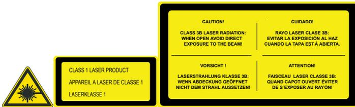
The digitizer is a Class 1 Laser Product. It uses one laser diode of a 80 mW type, classification class IIIb, wavelength 640-670 nm. The laser beam's deflection frequency is 80 1/s up to 170 1/s. The laser beam divergence is 12mrad.
