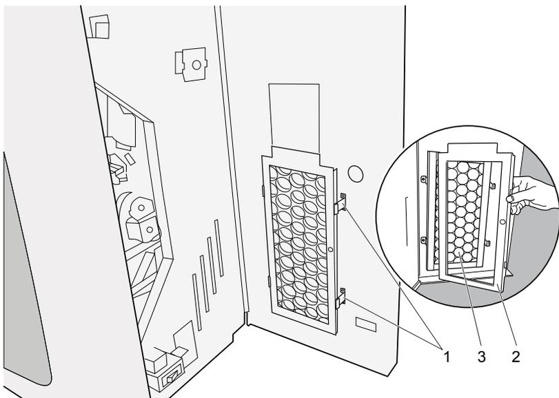
6. Remove the old air-filter element (3).
