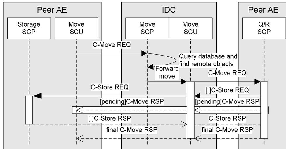
**Figure 2-10: Proxy C-Move Forward Sequencing of Activity**
