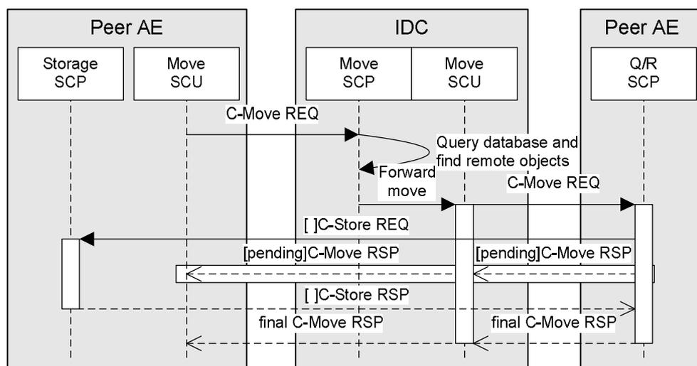
Figure 2-9: Direct C-Move Forward Sequencing of Activity
