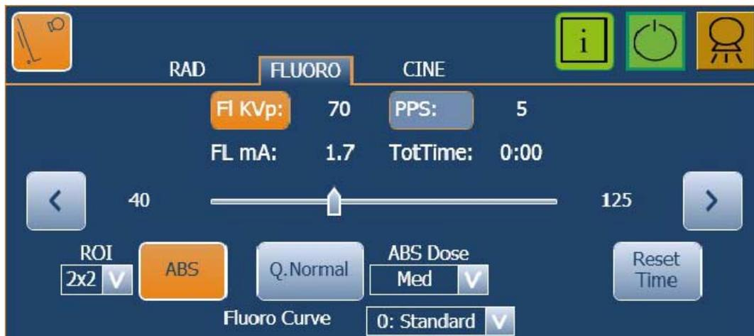
**FLUORO kVp INCREASE / DECREASE:** Selects the X-ray Tube voltage in Manual mode (no ABS mode). Fluoro kVp value is increased or decreased by selecting the “Fluoro kVp” Display (which will be highlighted) and changing the value with the “Increase” or “Decrease” buttons.
