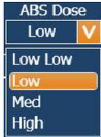
Once the “Quality Normal” is selected, the Dose per Frame can be set to Low-Low, Low, Medium or High depending on the image quality needed by the operator.
