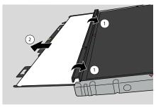
**5.** Put the black tray with the image plate onto the cassette, as shown in the figure below.
