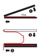
The design of the MAMORAY cassette ensures that the edge of screen and film are in close contact with the thoracic edge of the cassette. This way, the film draws closer to the thorax on closing the cassette and the distance between the edges of the film and the thorax side of the cassette can be limited to less than 2 mm.
