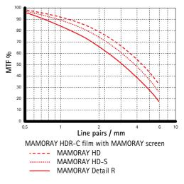
This curve is the result of measurements that give a degree of the "intrinsic" sharpness" of the film/screen system. This is a partial measurement of the total image quality of the film/screen system as perceived on the viewing box. The total image quality depends on other factors besides the "intrinsic sharpness". The principal factors are: graininess, noise, film contrast and aesthetic factors such as film density, image tint, etc.
