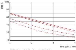
CURIX Ortho HT-L Plus film with CURIX Ortho screens
